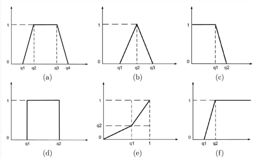
a) Trapezoidal function; b) Triangular; c) Left-shoulder; d) Crisp interval e) Linear f) Right-shoulder
