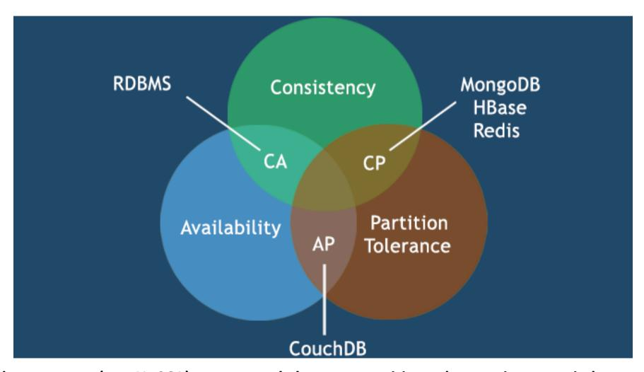
Modern systems (e.g. NoSQL) arose exactly because partition tolerance is a must in large-scale distributed systems
